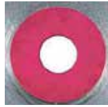
ruby type : enlargement of the nozzle orifice
