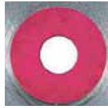
ruby type : enlargement of the nozzle orifice
